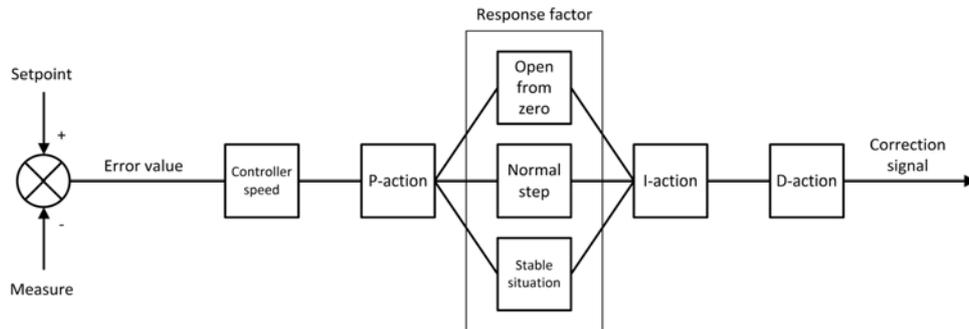
The controller speed controls the overall performance of the controller algorithm. Basically, to adjust the controller response, only the controller speed needs to be changed.
