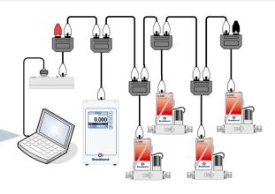
Example of a system using an RS232/FLOW-BUS interface for PC connection
