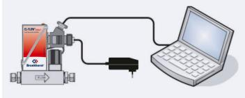
MFC directly connected to a PC via RS232  $\,$
